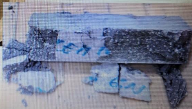
Fig. 3: Product of solidified sludge with 35% of DW in cement matrix with Nochar N910 after compressive strength test. – homogeneity
