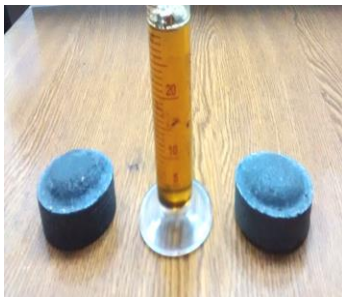
Oil Solidified with N910+ Encapsulated by Sulfur materials
