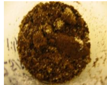
Sellafield Oil Sludge Solidification
